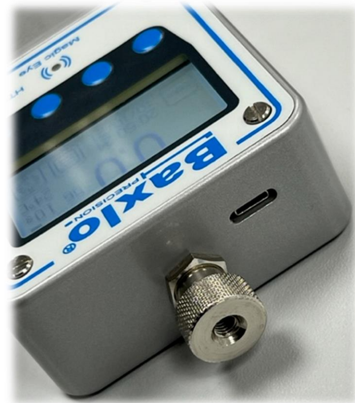
Detailed picture of the connections and the instrument clamping piece
