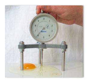
Our Baxlo Haugh tester will allow you to quickly and accurately determine the quality of the coating of egg albumin. This micrometer allows you to perform the Haugh test, which is the most internationally used for determining the freshness of the egg.
